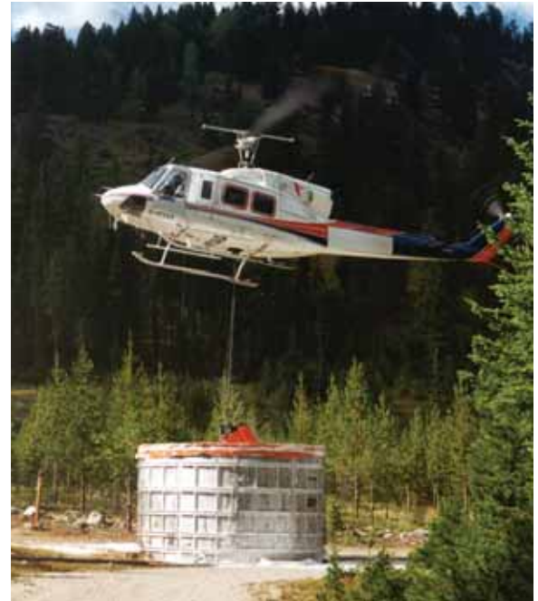
The Heliwell can fill a 2600 USG Bambi Bucket completely full
