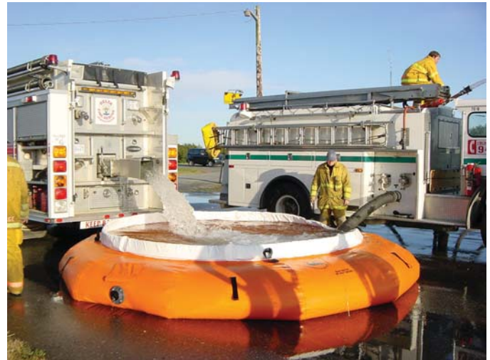
The Low-Profile tank can be easily filled by a water tender
