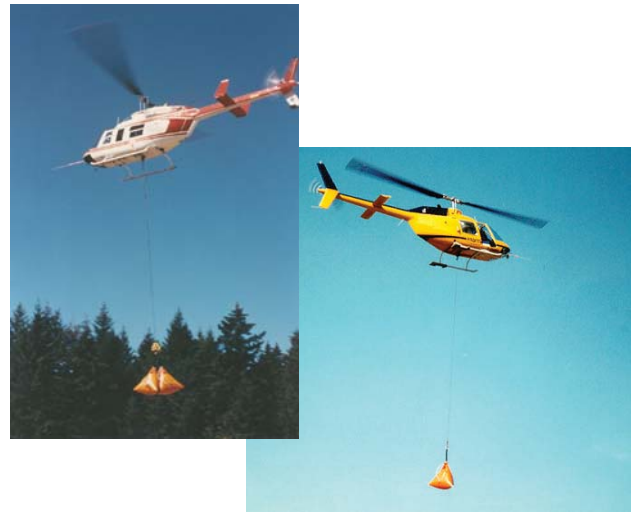
The Stilwell Flyer can be slung from helicopters in configurations of one or more
